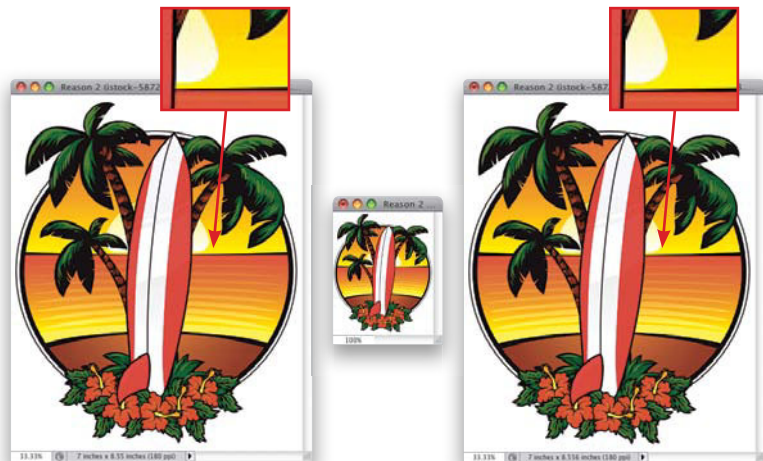
A Smart Object layer remains crisp when you resize it smaller then larger again
